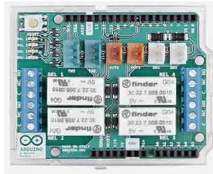
Arduino 4 Relay Shield
