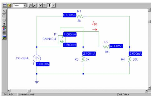
The current entering the right-hand node of the 10-k $\Omega$  resistor R2 is **Summary:** equal to 4.000 mA. Since this current is  $-i_{10}$ ,  $i_{10} = -4.000$  mA as found by hand.
