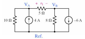
We note that after completing nodal analysis, we can find  $v_1$  as  $v_1 = V_A - V_B$ .
