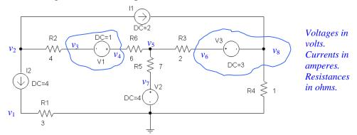
By inspection,  $v_7 = 4 \text{ V}$  and  $v_1 = (3)(4) = 12 \text{ V}$ .
