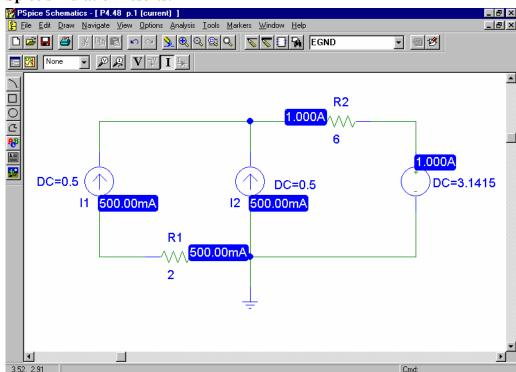
**Summary:** We see from the labeled schematic above that our choice for  $I_1$ ,  $I_2$  and  $V_1$  lead to 1 A through the 6- $\Omega$  resistor, or 6 W dissipated in that resistor, as desired.
