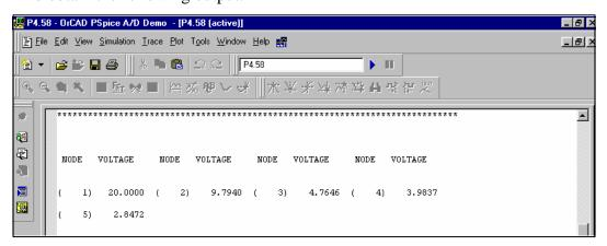
We see from this simulation result that the voltage  $v_5 = 2.847 \text{ V}$ .
