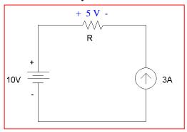
Choose R so that 3R = 5; then the voltage across the current source will be 5 V, and so will the voltage across the resistor R.
