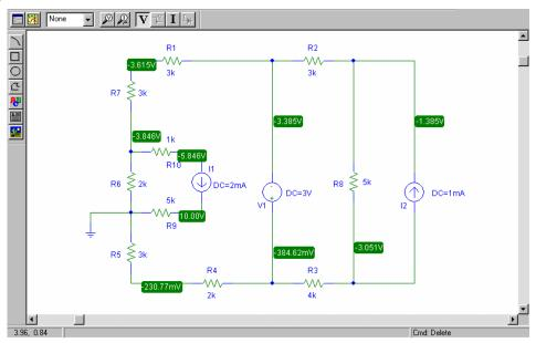
Again arbitrarily selecting the "+" reference as the top node of the 2-mA current source, we find the voltage across it is -5.846 - 10 = -15.846 V, in agreement with our hand calculation.
