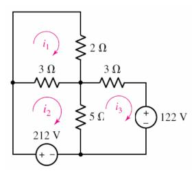
(a) The current through the 2  $\Omega$  resistor is  $i_1$ .
