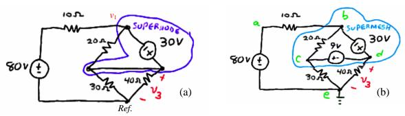
(a) We begin by noting that it is a voltage that is required; no current values are requested. This is a three-mesh circuit, or a four-node circuit, depending on your perspective. Either approach requires three equations.... Except that applying the supernode technique reduces the number of needed equations by one.
