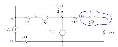
By inspection,  $v_4 = 4 \text{ V}$ .
